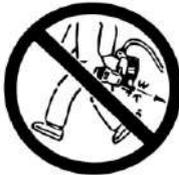
Do not pull trigger or depress contact arm while connected to the air supply as the tool may cycle, possibly causing injury.
