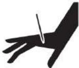
Keep hands and body away from the discharge area of the tool. A contact arm tool may bounce from the recoil of driving a fastener and an unwanted second fastener may be driven possibly causing injury.
