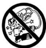
**DO NOT USE OXYGEN, COMBUSTIBLE GASES, OR BOTTLED GASES AS A POWER SOURCE FOR THIS TOOL AS TOOL MAY EXPLODE, POSSIBLY CAUSING INJURY.**
